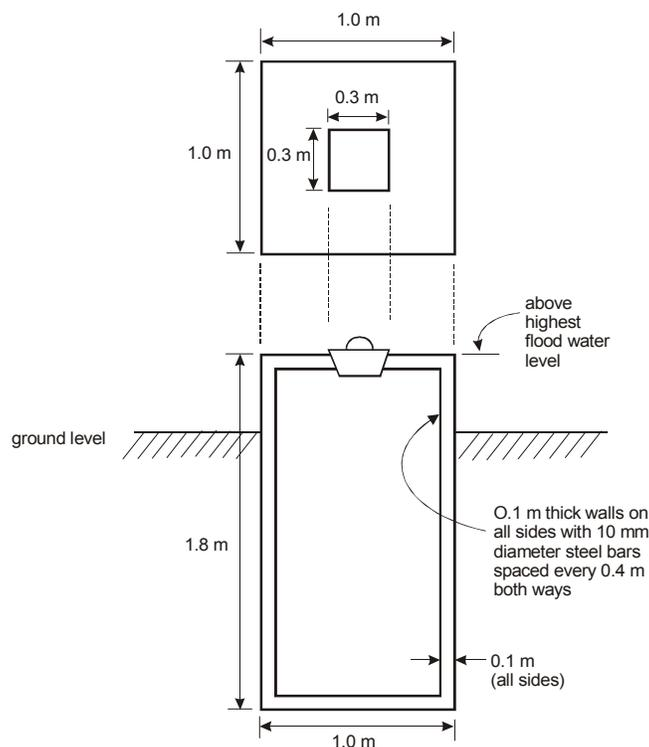
Figure D. Concrete Septic Vault
