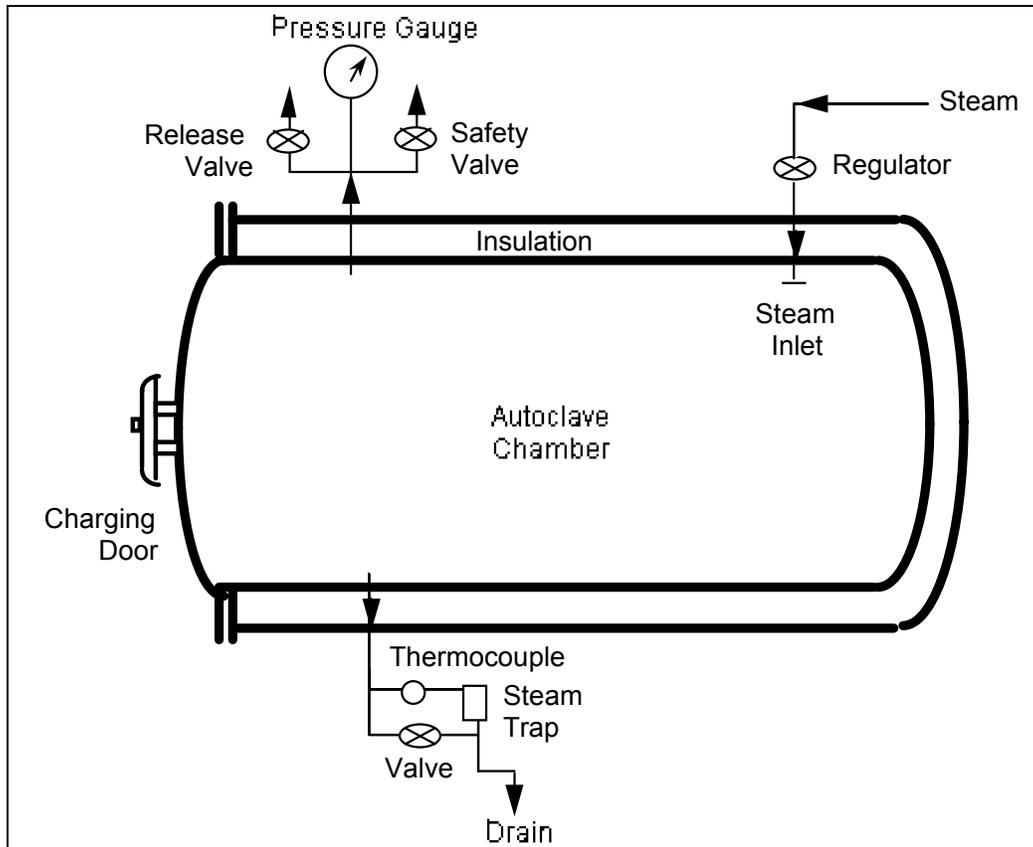
**Figure 6. Typical Autoclave Treatment System**
