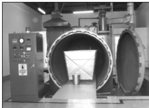
Figure B. Autoclave Treatment System (PAE Environmental, Inc.)
