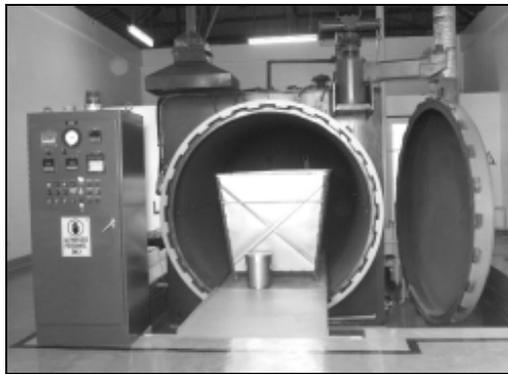
Photograph 16. PAE Autoclave System
