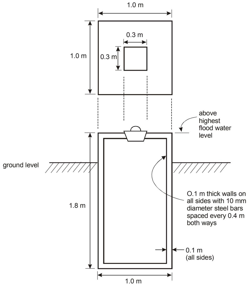
**Figure 7. Basic Concrete Septic Vault Design**
